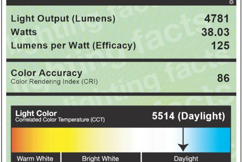
All results are according to IESNA LM-79-2008: *Approved Method for the Electrical and Photometric Testing of Solid-State Lighting.* The U.S. Department of Energy (DOE) verifies product test data and results.
